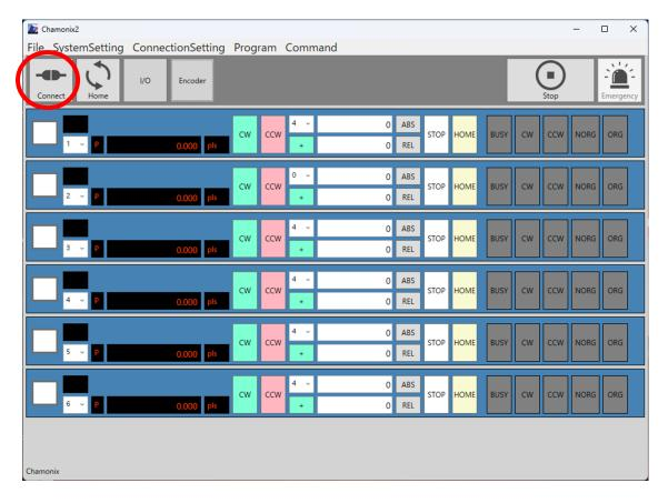
Press the "Connect" button to confirm and initialize the connection.
