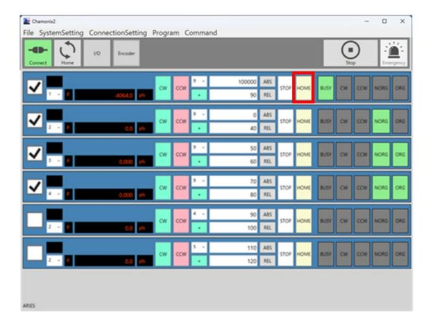
To return to the origin, it is also possible to return to the origin of only a specific axis by clicking the "HOME" button on the individual axis.
