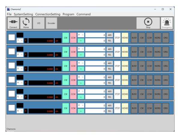
Here is an example of the screen of Chamonix 2 when it is first launched. The default communication interface is "RS-232C", and the RS-232C setting is set to "COM1" and the baud rate is "115200baud" for the COM port by default.
