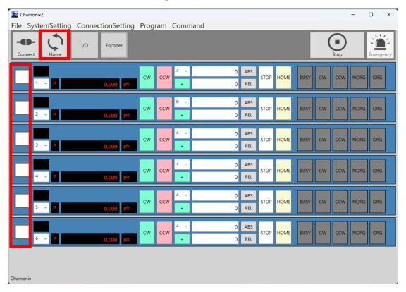
When you press "Return to Origin", the checked axis in the red frame will return to the original point.
