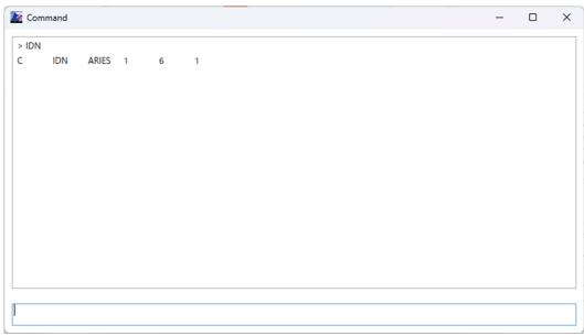
Enter a command in the send box and press "Enter" to send it to the controller. The STX  $^{12}$  header and CRLF  $^{13}$  delimiter required for RS-232C communication are automatically added.
