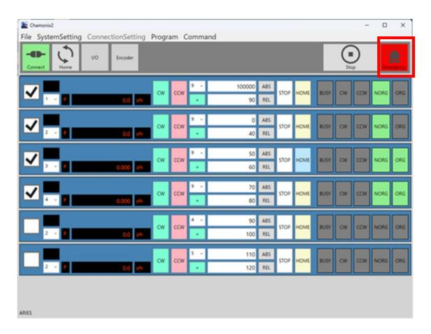
When an emergency stop signal is received, "Emergency Stop" lights up red.
